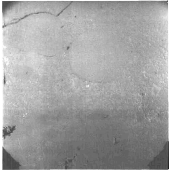
Figure 3. Scanning electron microscope backscattered-electron image of amygdaloidal volcanic rock. Small brighter patch in center of image is composed of Y-HREE-Zr minerals. Field of view is approximately 4 mm.
