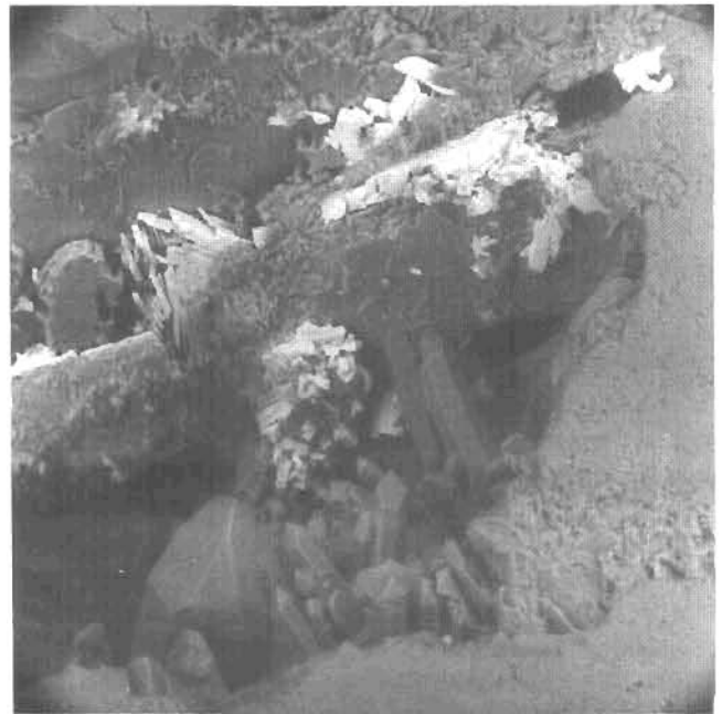
⇒ Figure 7. Scanning electron microscope backscattered-electron image of REE minerals (bright) and quartz crystals (dark) around a "thunder egg" vug. Field of view is approximately 0.7 mm.
