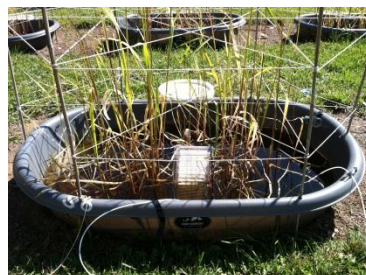
Figure 5. Mesocosms with wild rice populations subject to different sulfate concentrations. A peeper used to sample sulfate, sulfide, and iron concentrations in the sediment profile is in the middle of the mesocosm.
