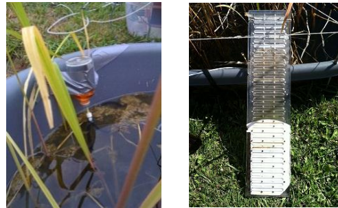
Figure 6. Microelectrodes (right) and pore water sippers (left) for investigating speciation of sulfur and iron concentrations in sediment profiles.
